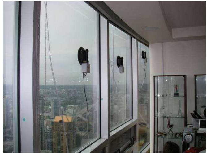
Figure B9: Pressure gauges mounted on suction cups, with tube attached to IGU desiccant tube, suite 3903.
