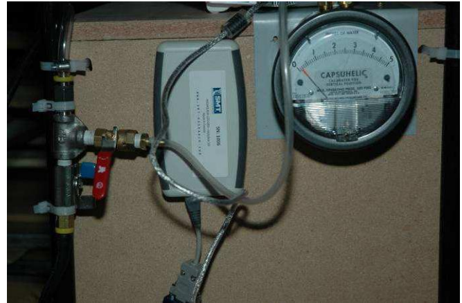
Figure B5: Pressure testing apparatus including valves and Capsuhelic analog gauge back-up.
