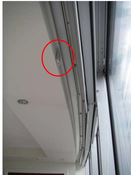
Figure D2: Location of installed data-logger, behind curtains at ceiling valence.
