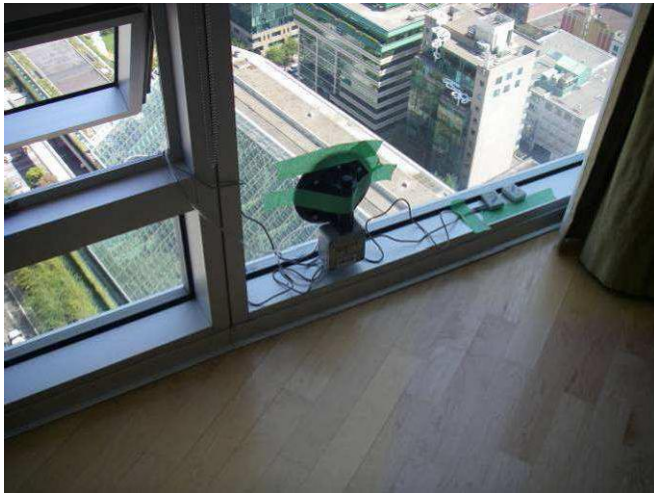
Figure B10: Pressure gauge mounted on suction cup, with tube attached to IGU desiccant tube, suite 4502.
