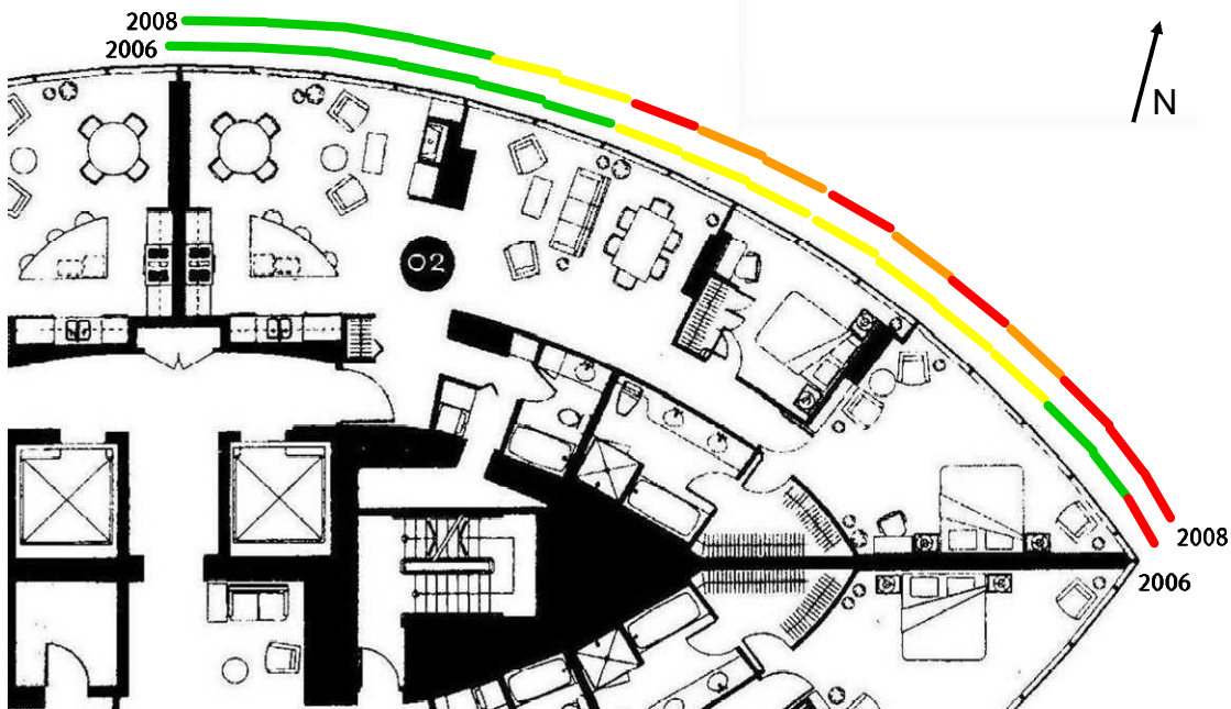
Figure A11: Suite 4502, Degradation of IGU Condition between February 2006 and August 2008 (18 months).
