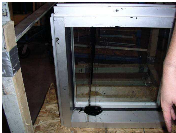
Fig. 3.8.1 In-Situ Repair Mock-up After Sealant Injection
