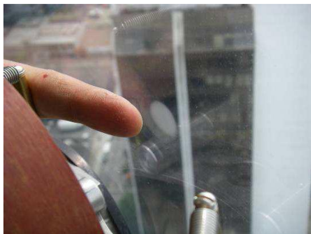
Fig. 3.2.3 Dewpoint Test Apparatus and Condensation on Surface #5 Indicating the IGU airspace Dewpoint Temperature
