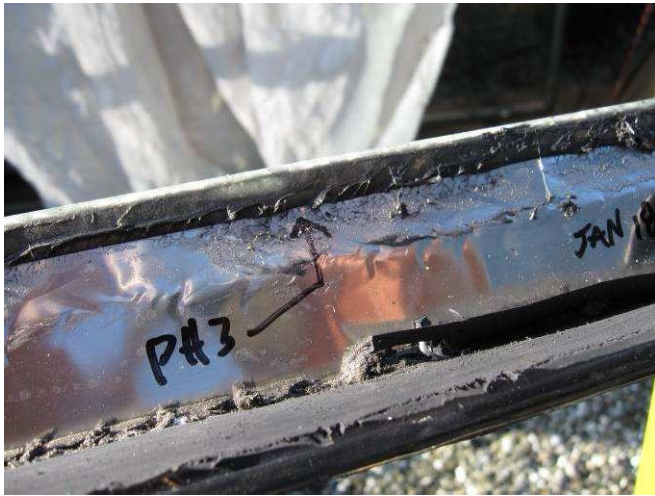
Fig. 3.7.1.5 Typical Buckling of stainless steel edge band of IGU 44774.
