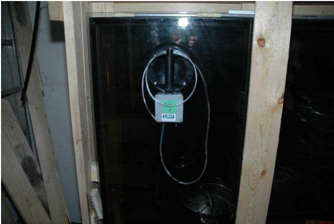
Figure B4: Wireless pressure sensor WiDAQ attached to Visionwall IGU using glazing suction cup.
