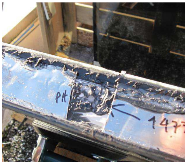
Fig. 3.7.1.2 Edge band removed at ripple revealing open joint between PVC and aluminum extrusion spacer bar components
