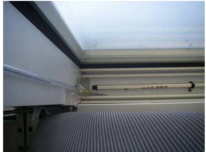
Figure B11: Pressure gauge tube attached to desiccant tube IGU tube.
