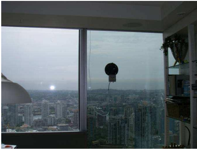
Figure B8: Pressure gauge mounted on suction cup, with tube attached to IGU desiccant tube, suite 3903.
