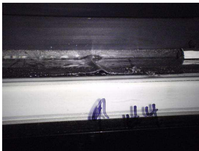
Fig. 3.7.1.4 Typical ripple or "fish mouth" in the stainless steel edge band of IGU 43882.
