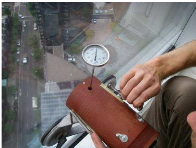
Fig. 3.2.2 Dewpoint Test Apparatus and Condensation Indicating Dewpoint Temperature
