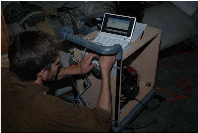
Figure B2: Pressure testing apparatus consisting of compressor and BiG mini-laptop.
