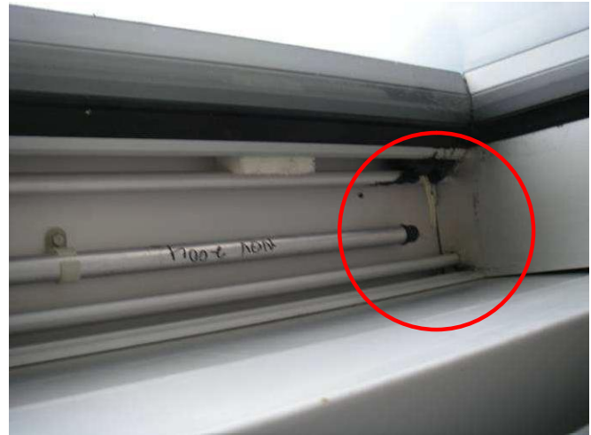
Figure B7: Desiccant tube attached to IGU through 1/8" clear flexible tubing. Desiccant tube is removed from IGU to all connection of pressure gauge.
