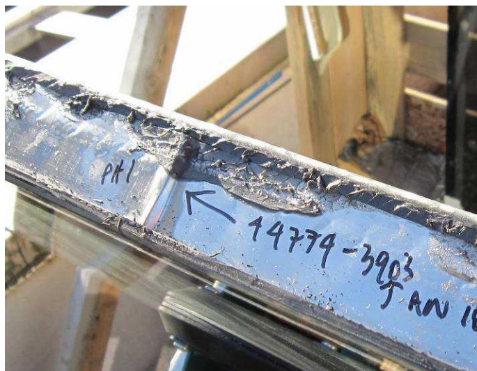
Fig. 3.7.1.1 Typical ripple or "fish mouth" in the stainless steel edge band. IGU 44774
