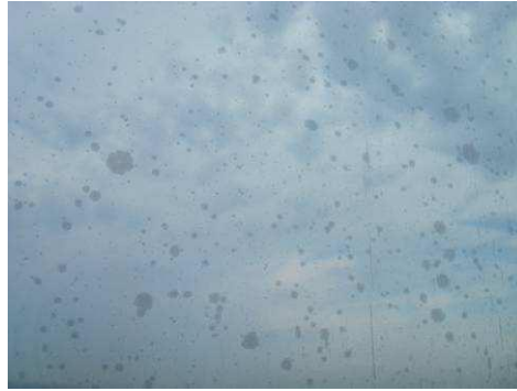
Large low-e corrosion spots visible from 3m
