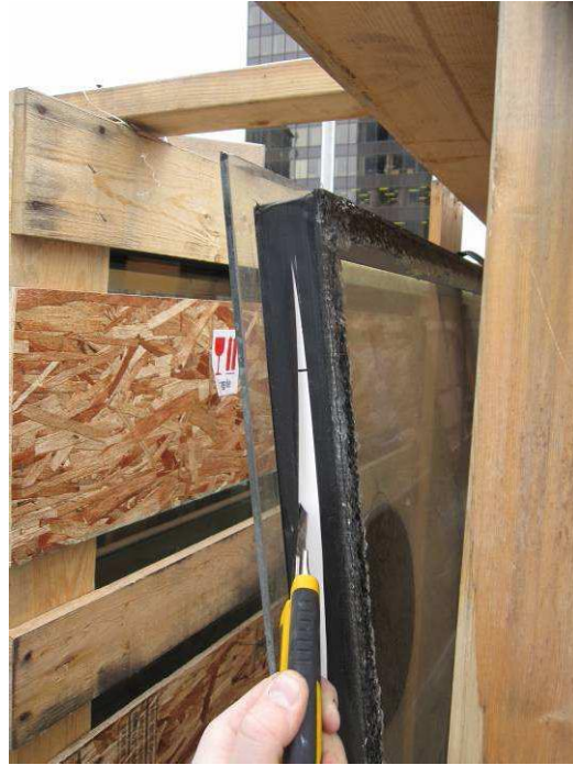
Figure E93: Stainless Steel foil is covered with a black thermosetting sealant, but is not adhered to the vinyl spacer bar.
