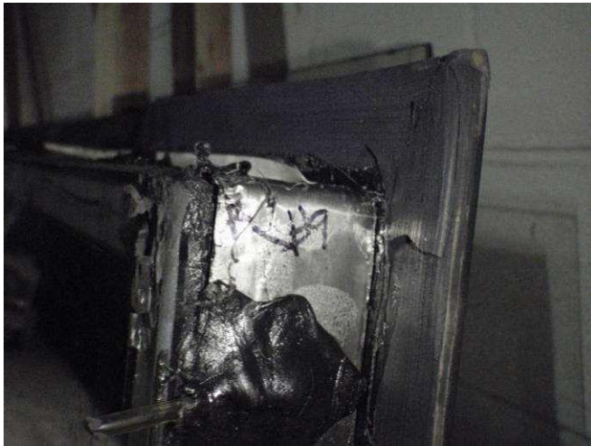
Figure E86: Stainless steel edge band discontinuity #9 at corner.
