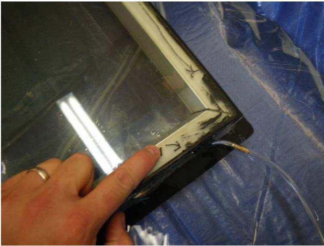
Figure E44: Injecting air into IGU through desiccant tube using air-compressor.
