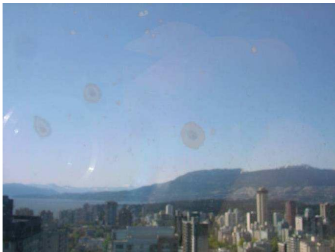
Figure F31: Suite 3101, May 15, 2008, low-e corrosion spots on glass surface #2.
