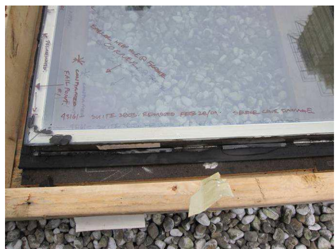
Figure E38: Discontinuities in edge seal noted an lower sill of IGU.
