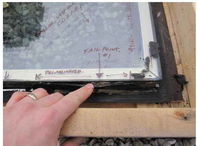
Figure E36: Discontinuities in edge seal noted at lower left corner of IGU.
