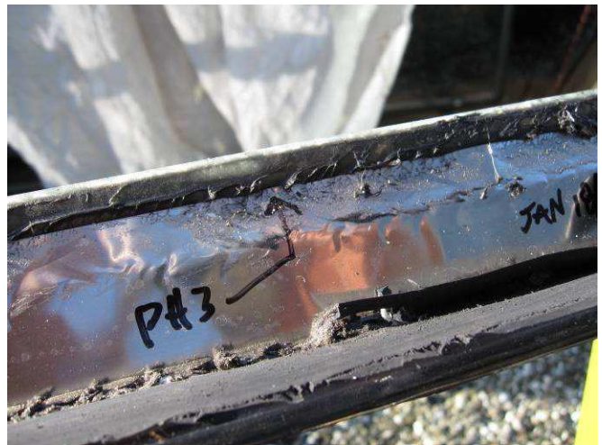
Figure E9: Buckling of stainless steel edge band (edge seal discontinuity PH3).
