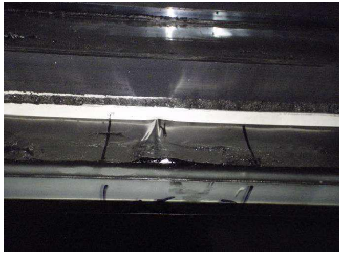
Figure E77: Stainless steel edge band discontinuity #5.
