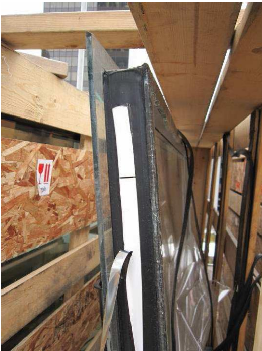
Figure E94: Gap in vinyl extrusions between corner and edge pieces allow air leakage directly into IGU should the perimeter edge seal be compromised (i.e. nicked during installation or at seal details).
