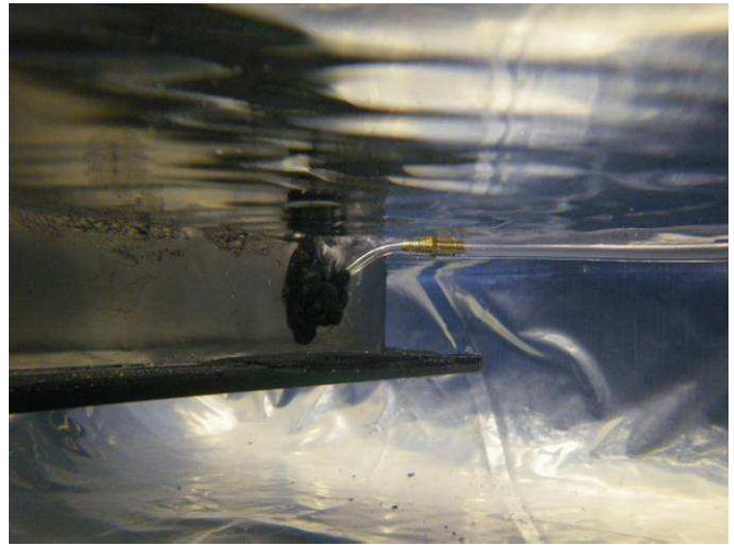
Figure E51: Desiccant tube used for pressurization during test, small leak through sealant around tube (#11). Note that sealant may have been damaged during removal of the IGU.
