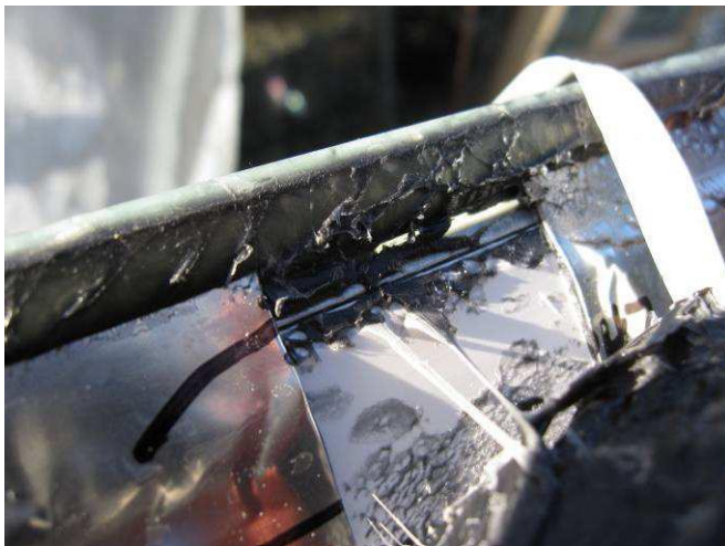
Figure E8: Close-up of buckled of stainless steel edge band (edge seal discontinuity PH2). Stainless steel edge seal cut away revealing sealant and vinyl/aluminum spacer joint.
