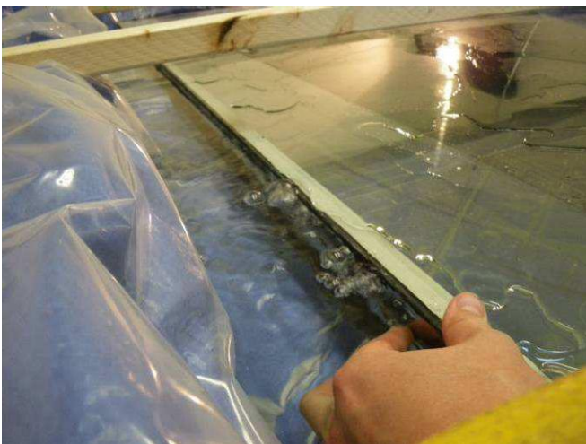
Figure E48: Edge seal discontinuities #6 and #7.
