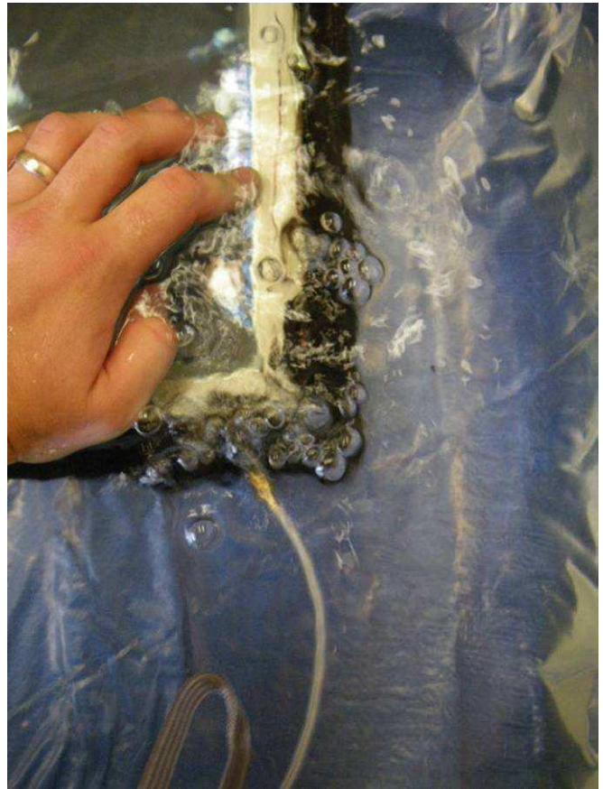
Figure E53: Discontinuities #9,11,12,13,14 at upper right corner of IGU.
