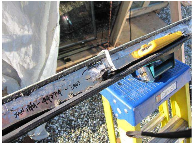
Figure E8: Buckling of stainless steel edge band (edge seal discontinuity PH2). Stainless steel edge seal cut away revealing sealant and vinyl/aluminum spacer joint.
