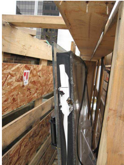
Figure E97: Edge of foil wrapped and sealed as shown in Figure E99.
