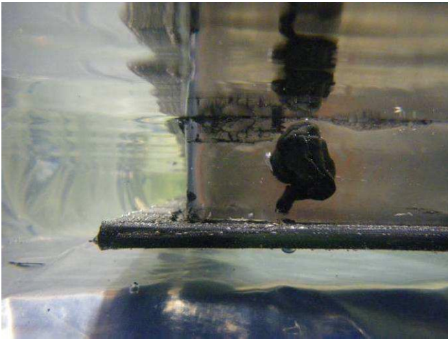
Figure E50: Edge seal discontinuity #7 (foreground) and #6, viewed underwater during test.
