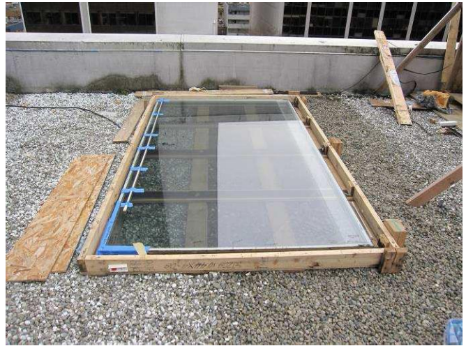
Figure E40: Overview of failed IGU 43161 prior to crating up for laboratory testing.
