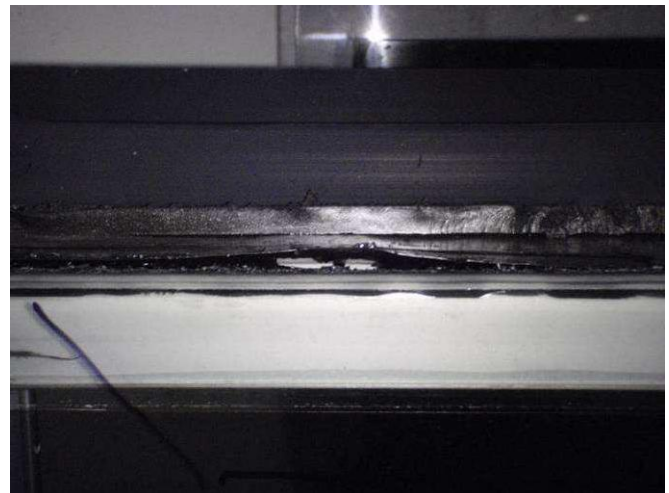
Figure E71: Stainless steel edge band discontinuity #2.
