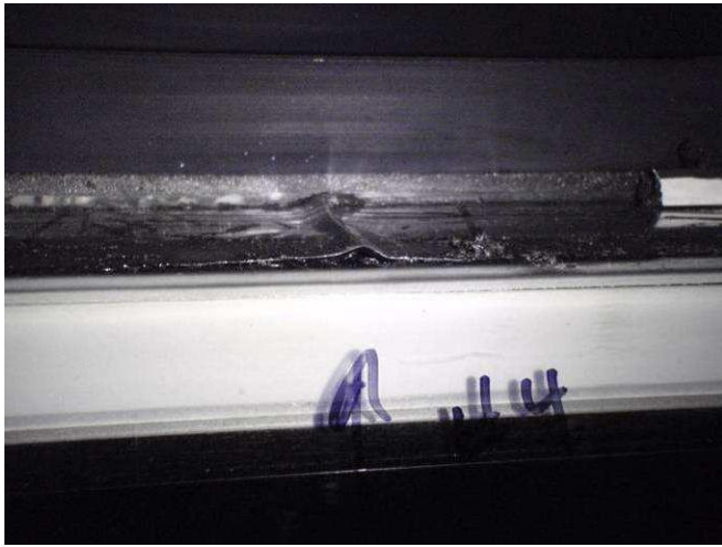
Figure E74: Stainless steel edge band discontinuity #4.
