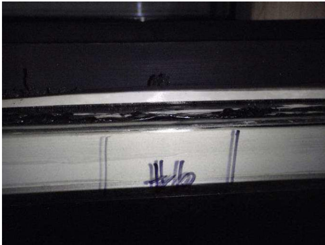
Figure E78: Stainless steel edge band discontinuity #6.
