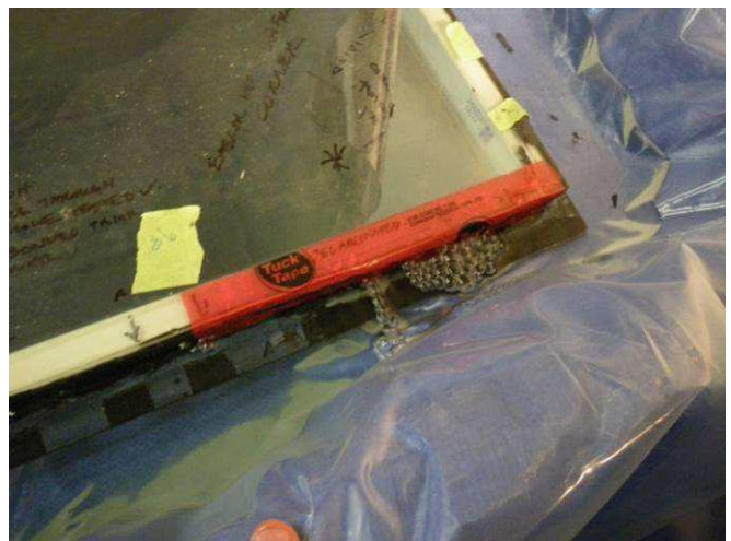
Figure E49: Edge seal discontinuity #1, continues to leak a small amount of air while sealed.
