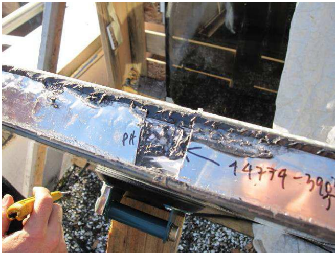
Figure E7: Buckling of stainless steel edge band (edge seal discontinuity PH1). Stainless steel edge seal cut away revealing sealant and vinyl/aluminum spacer joint.
