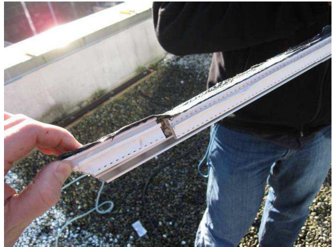
Figure E13: Vinyl extrusion edge spacer, note gap between components. Stainless steel spacer therefore acts as the primary air/vapour/moisture IGU seal.
