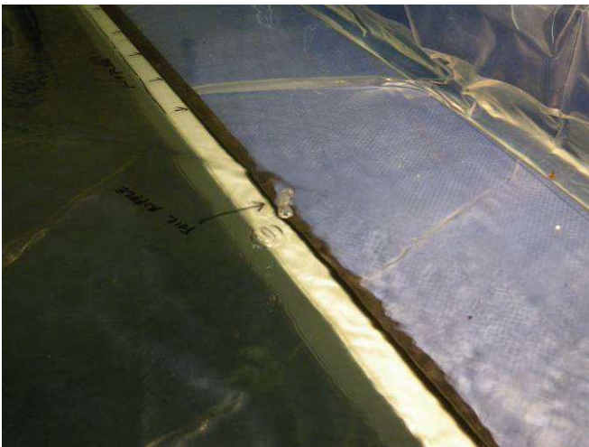
Figure E58: Discontinuity #16 at left side of IGU.
