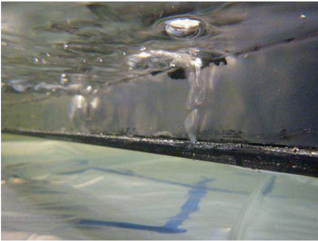
Figure E50: Edge seal discontinuity #7 (foreground) and #6, viewed underwater during test.
