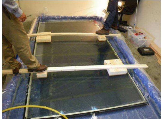
Figure E42: IGU Submerged under water during testing. IGU was buoyant and therefore had to be restrained under the water for the test.
