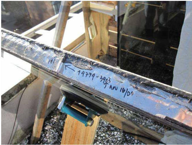
Figure E5: Buckling of stainless steel edge band (edge seal discontinuity PH1)
