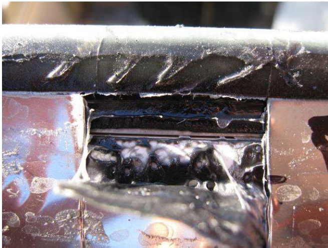
Figure E12: Buckling of stainless steel edge band (edge seal discontinuity PH4). Stainless steel edge seal cut away revealing sealant and vinyl/aluminum spacer joint, close-up.
