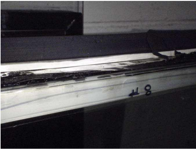
Figure E82: Stainless steel edge band discontinuity #8.
