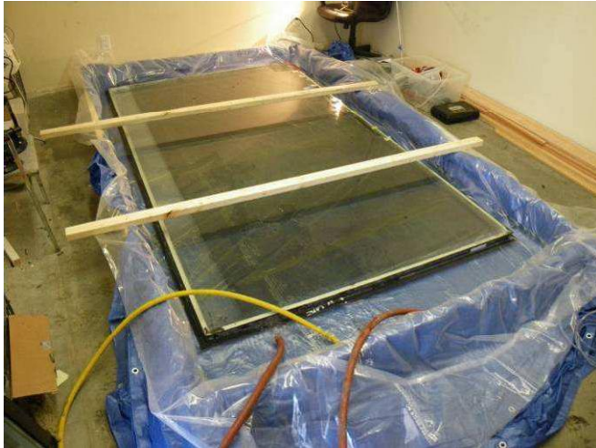
Figure E41: Unit 43161 setup within a water bath to locate edge seal discontinuities.
