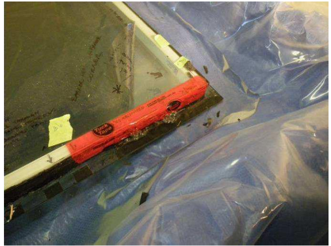
Figure E45: Lower left corner, largest visible discontinuity (#1) in foil. This obvious discontinuity was sealed with waterproof tape for first part of test to allow for IGU to be pressurized and locate other leakage paths.
