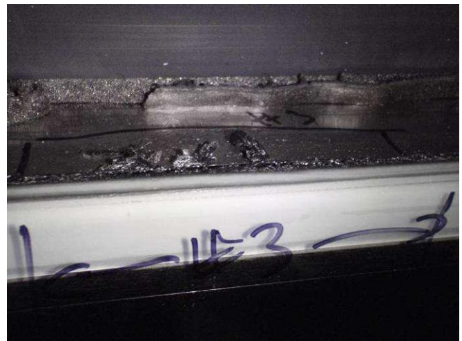
Figure E73: Stainless steel edge band discontinuity #3.
